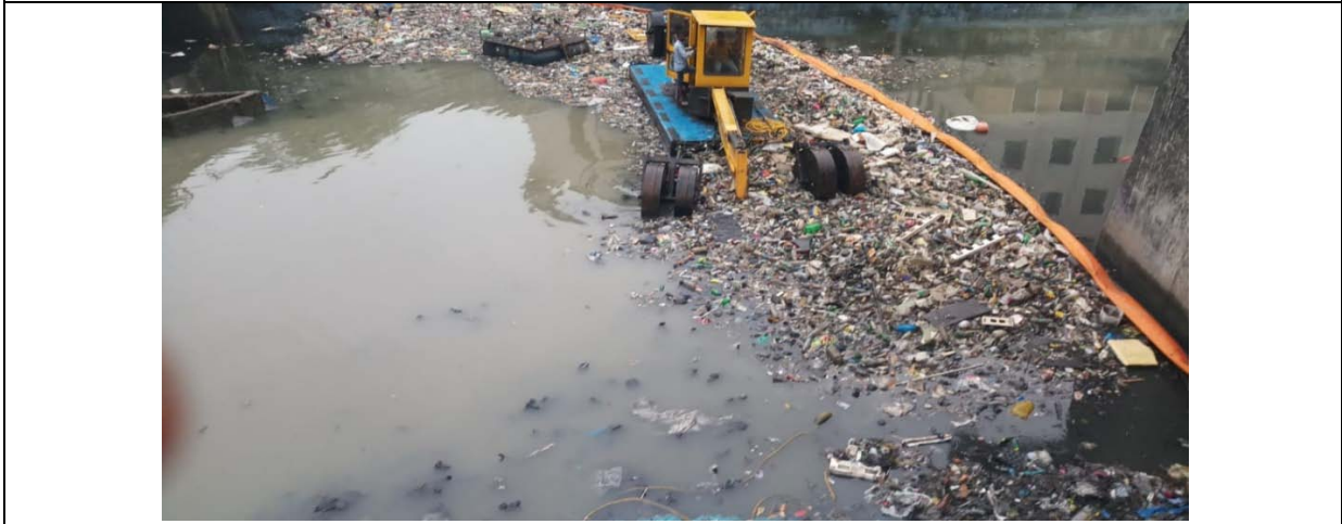
Trash Boom Machine for collection of Floating trash in rivers and mangroves
